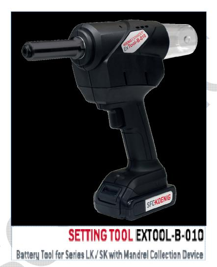
The new battery powered ExTool-B-010 provides the same efficient, high-performance capabilities found in our hydro-pneumatic ExTools. A rechargeable lithium-ion battery provides reliable power, eliminates the need for a pneumatic hose, and allows for mobile, flexible installation of the full line of SK and LK KOENIG EXPANDER plugs. The unit features the same maximum pulling force of other ExTool models.
